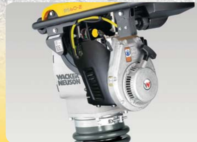
The slim design makes compacting in trenches more comfortable.
